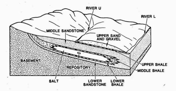
Figure 3.1.1. Schematic Diagram of the Reference Site. One side of the symmetric basin is shown. The upper end of the valley is approximately elliptic with the repository located on the minor axis; the sides of the valley are parallel below the repository. The vertical exaggeration of scale is approximately 20. -
