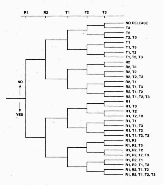
Figure 2.4.1. Potential Combinations of Two Release and Three Transport Phenomena
