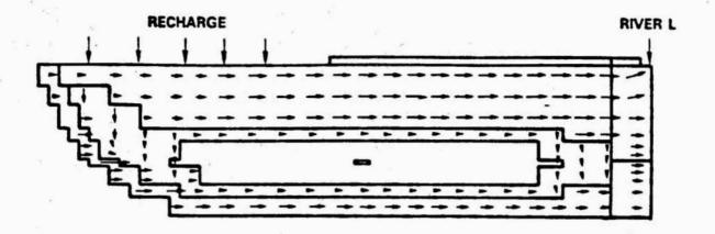
Figure 3.2.5. Fluid Velocity Vectors of the Reference Site
